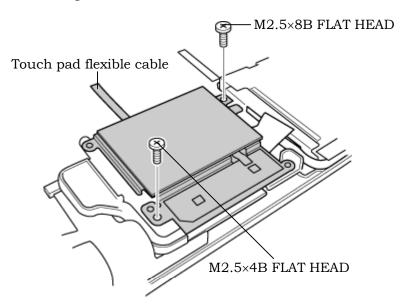
Figure 4-21 Removing the touch pad
